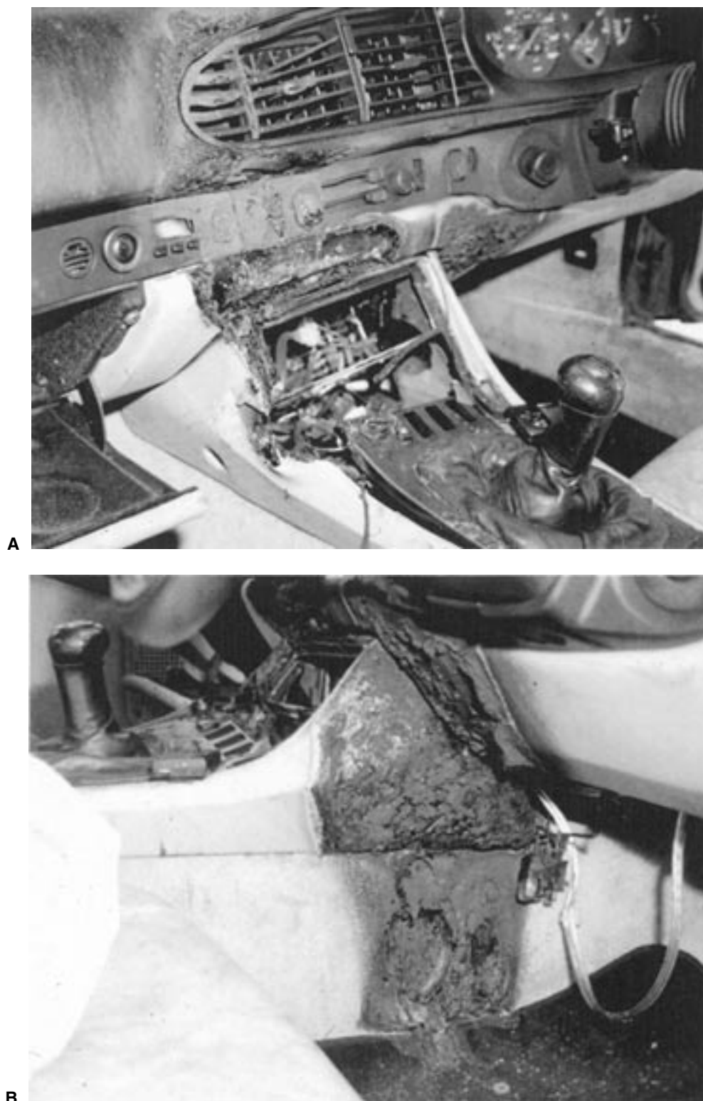
FIG. 1a, 1b—Areas of burning around front console of motor vehicle.
